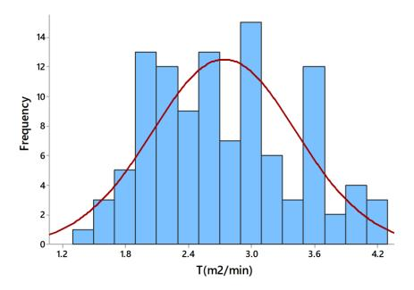
**Figure 3.** Histogram For Tazerbo wellfield Aquifer Transmissivity T (m<sup>2</sup>/min).
