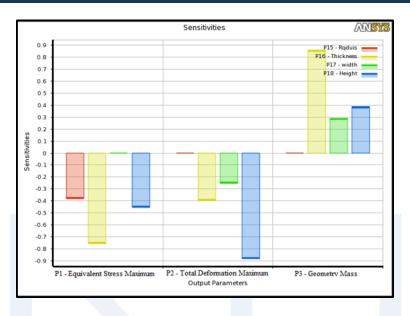
Figure 8: Sensitivities of the objective function and the constraints to design variables
