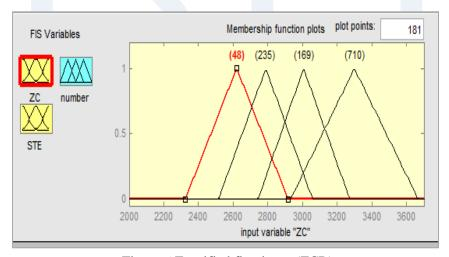
Figure 6.Fuzzified first input (ZCR)
