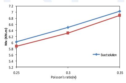
Figure 12. Bending moment (Mx)-Poisson's ration (v) relationship (case two)
