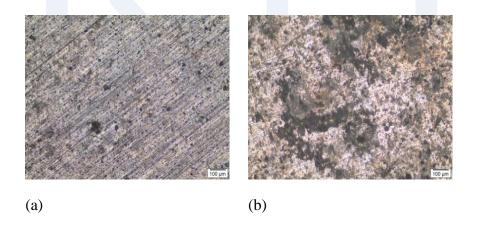
Figure 8. Optical micrograph of composites containing of MgAl - % 5 Mo<sub>2</sub>C, sample sintered at 400 °C for 5 minutes ,(a)before corrosionand (b)after corrosion
