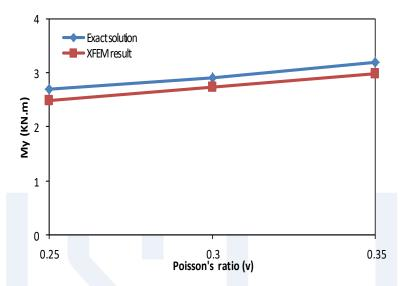
Figure 13. Bending moment (My)-Poisson's ration (v) relationship (case two)
