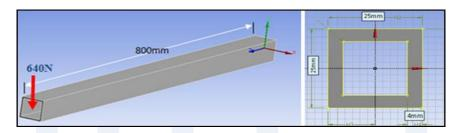
Figure 6: Boundary conditions and initial geometry constraints of the beam.
