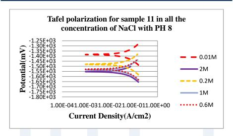
Figure 3. Tafel Polarization of Mg AL alloys at different concentrations in Na Cl solution with pH = 8.
