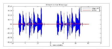
Figure 3. Short time energy of a speech signal sample
