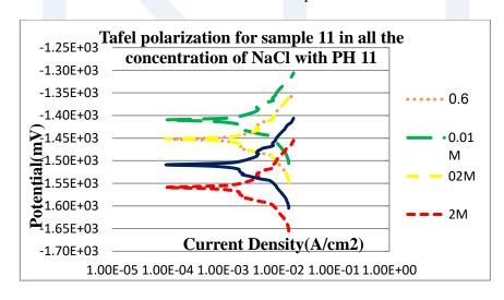
Figure 4. Tafel Polarization of Mg AL alloys at different concentrations in NaCl solution with pH=11
