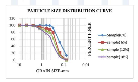
Figure 3: Grain size distribution for the tested soil
