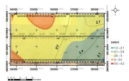
**Figure 8**. Interpolation Surface and Contour Maps For Tm<sup>2</sup>/min Using (IDW).
