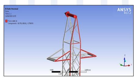
Figure 6: Direction of acting wind pressure
