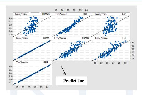
$\label{eq:Figure 4.Comparison Between The Predicted and Measured Tazerbo} Wellfield Aquifer Transmissivity T m^2/min \ .$
