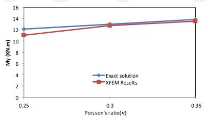
Figure 10. Bending moment (My)-Poisson's ration (v) relationship (case one)
