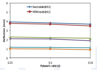
Figure 11. Deflection--Poisson's ration (v) relationship at different thickness (case two)
