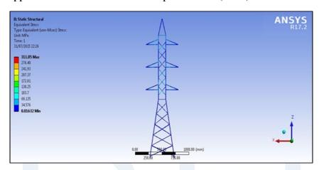
Figure 8: Equivalent Von-Mises stress across tower
