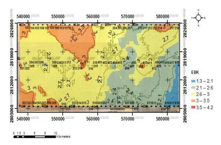
**Figure 6**. Interpolation Surface and Contour Maps For Tm<sup>2</sup>/min Using (EBK).
