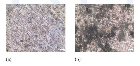
Figure 6. Optical micrograph of composites containing of Pure MgAl) sample sintered at 400 °C for 1 inute,(a)before corrosionand (b)after corrosion
