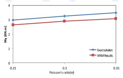
Figure 16. Bending moment (My)-Poisson's ration (v) relationship (case three)
