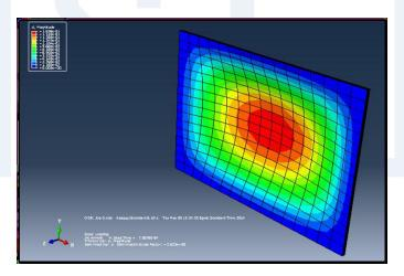
Figure 7. Crack Propagation of simply supported plate (ABAQUS/CAE)
