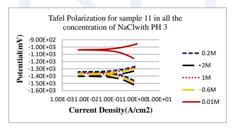
Figure 2. Tafel Polarization of  $\mbox{ Mg AL}$  alloys at different concentrations  $\mbox{Na Cl}$  solution with  $\mbox{pH}=3$
