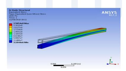
Figure 7: Equivalent stress distribution for the initial set.
