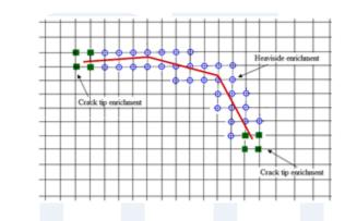
Figure 1. The nodes enriched with the Heaviside and crack tip enrichment functions
