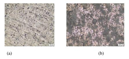
Figure 7. Optical micrograph of composites containing of MgAl-% 2.5 SiC, sample sintered at 400 °C for 3 minutes,(a)before corrosionand (b)after corrosion
