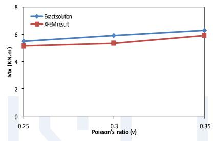
Figure 15. Bending moment (Mx)-Poisson's ration (v) relationship (case three)
