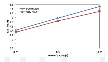
Figure 9. Bending moment (Mx)-Poisson's ration (v) relationship (case one)
