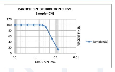
Figure 1: Grain size distribution for the tested soil
