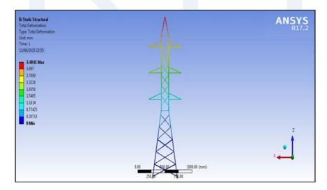
Figure 7: Total deformation across tower
