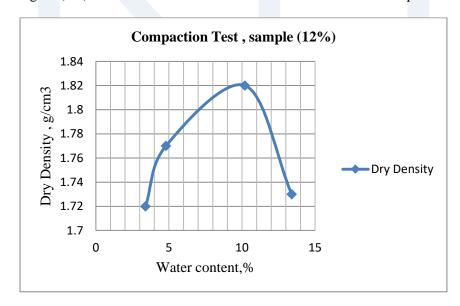
Figure (4-b)- the results obtained from Standard Proctor Test – sample \$12%\$
