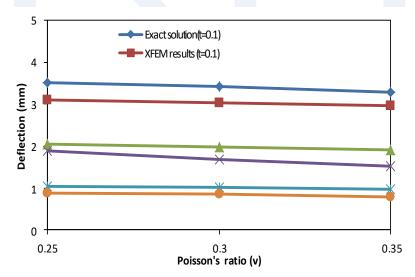
Figure 14. Deflection--Poisson's ration (v) relationship at different thickness (case three)
