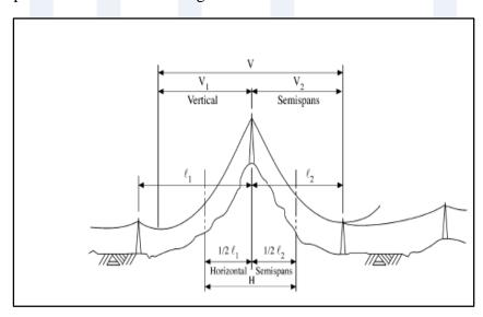
Figure 1: Vertical design span is the distance between low points of adjacent spans and is indicated.
