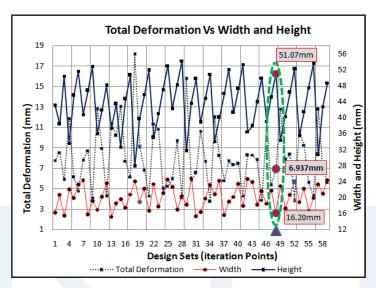
Figure 7: Maximum deformation and beam cross section versus design sets.
