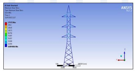
Figure 9: Maximum shear stresses across tower
